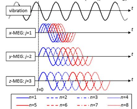
**Fig. 1:** MEG arrangement relative to the mechanical actuation signal in SLIM-MRE. For better visualization, only one MEG-cycle is illustrated per component and time step  $n$ . The start of all MEGs in the first time step ( $n=1$ ) coincides with  $t=0$ . Using  $f=5$ kHz, the sampling interval with respect to the start time of the  $x$ -,  $y$ - and  $z$ -MEG corresponds to 25  $\mu$ s, 50  $\mu$ s and 75  $\mu$ s, respectively.
