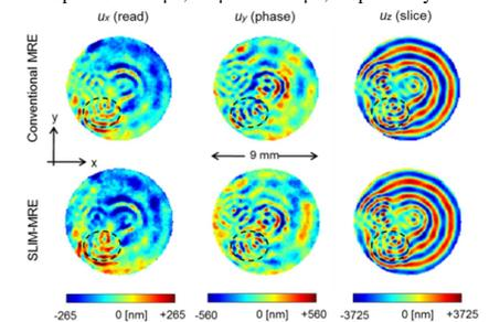
**Fig. 2:** Complex wave images in the axial plane at 5 kHz acquired using conventional MRE (top) and using SLIM-MRE (bottom). One displacement component is shown per column as indicated in the heading. The ROI is demarcated with dashed lines.
