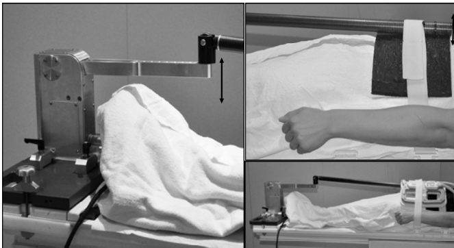
Fig.1: Proposed nonmagnetic driver system for abdominal MRE. A close view of the driver which is placed at the end of the patient table is shown in the left image. A carbon fiber rod is mounted to the horizontal lever arm for efficient wave transmission to the transducer mat (shown in the upper right image). The entire setup is shown in the bottom right figure. The vibration direction is indicated by arrows.
