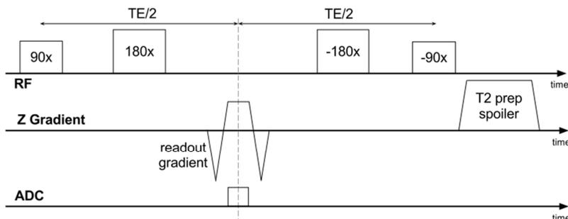
Figure 1. Pulse sequence diagram of a 2-MLEV T2 prep with a fully balanced readout gradient along the z-axis inserted at the midpoint. The readout gradient need not to be on z-axis only. Also note that its duration and those of the RF pulses are exaggerated for illustration purposes.
