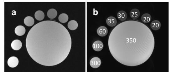
Figure 2. a) Phantom imaged while stationary using bSSFP without T2 prep, and b) with T2 prep of TE=20ms. T2 values as measured by another standard T2 mapping sequence are labeled.
