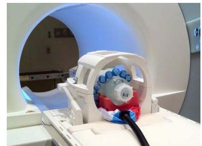
Figure 4. The T2 phantom displaced pneumatically during imaging to mimic respiratory motion
