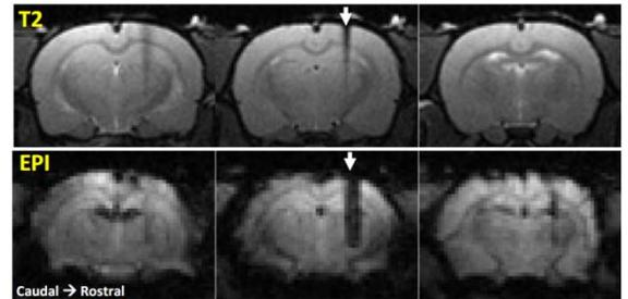
Figure 2: Tungsten electrode caused limited MR susceptibility distortion (arrow)
