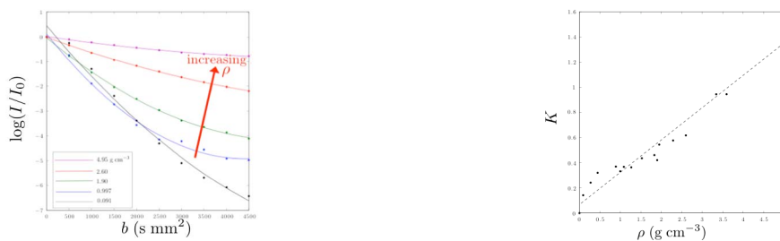
Figure 2: Left panel: A selection of signal attenuation curves for the test object. Each curve represents a different concentration of colloids as indicated in the key. Right panel: The kurtosis K as a function of colloidal concentration \rho for the various samples that comprise the isotropic test object. A basic linear fit allows us to extrapolate the surface area of barriers required for a given kurtosis.
