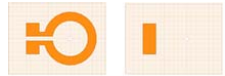
Figure 1 Model of the flexible resonator: Loop and capacitor plates (top metal - left), capacitor plate (bottom metal - right)
