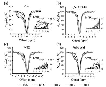
**Figure 2.** CEST z-spectra acquired at 11.7T of 10 mM (a) glutamate (Glu), (b) 3,5-DFBGlu, (c) methotrexate (MTX) and (d), folic acid in PBS at varying pH and at 37°C. ( $MTR_{assym} = (M_{-\Delta\omega} - M_{+\Delta\omega}) / M_b$ , where  $M_{-\Delta\omega}$  and  $M_{+\Delta\omega}$  represent the bulk water signals acquired with selective RF saturation at  $\pm\Delta\omega$  resonance offset from the water frequency)
