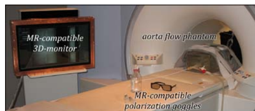
Fig. 1: Setup of the aorta flow phantom experiment. The MR-compatible 3D-monitor with the polarization goggles was operated near the magnet's bore.
