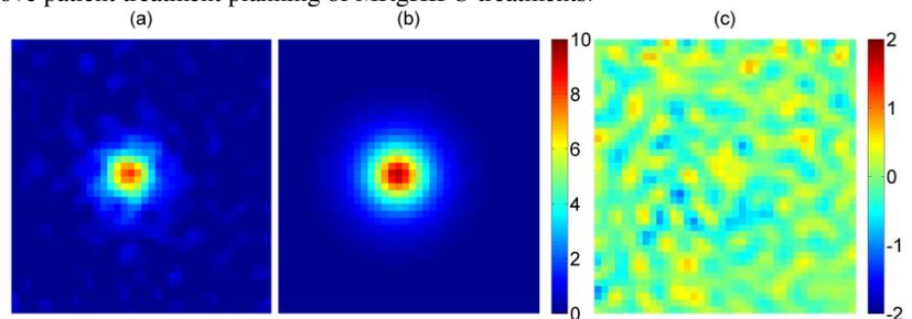
**Figure 4:** (a) Experimental temperatures in a 2x2 cm<sup>2</sup> region at the end of heating, (b) Fitted temperatures from Eq. 1, (c) Difference between fitted and experimental temperatures.
