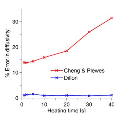
**Figure 2:** Diffusivity estimation results for simulations with varied heating times.
