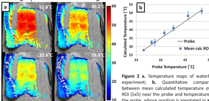
**Figure 2** a. Temperature maps of waterbath experiment; b. Quantitative comparison between mean calculated temperature of an ROI ( $5 \times 5$ ) near the probe and temperatures of the probe, whose position is annotated in a.
