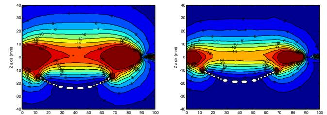
Fig. 4: Magnetic field map of the in-house coil in air (left), and after tuning for use in water (right). The scale has been altered to adapt the increased signal intensity
