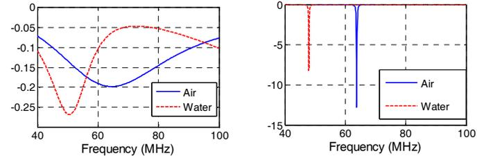
Fig. 2: S11 response from the simple coil (left) and in-house coil (right) in the different scenarios.
