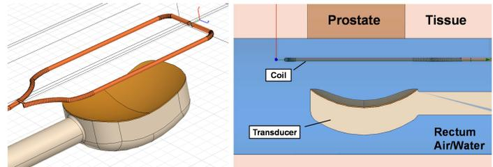
Fig. 1: Simple endorectal coil with HIFU transducer (left) and a cross plane cut of the simulation environment (right).
