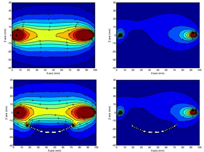
Fig. 3: Magnetic field map through the center of the simple coil for air (top left) and water (top right) when the transducer is not present, and in air (bottom left) and water (bottom right) when it is.
