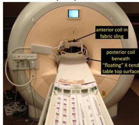
Figure 1. Setup of the X-tend tabletop.
