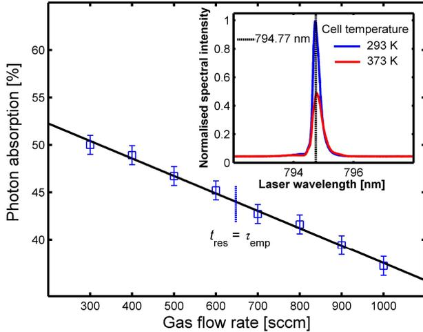
**Figure 2:** Inverse linear dependence of photon absorption with gas flow rate. The black line is a linear fit to experimentally measured photon absorption percentage using  $(P_{\text{cold}} - P_{\text{hot}})/P_{\text{cold}}$  and the vertical blue line indicates the absorption for which the cell residency time,  $t_{\text{res}}$  is equal to the spin exchange time,  $\tau_{\text{emp}}$ . Inset shows absorption spectrum (red) for gas flowing at 300 sccm through a cell at  $T = 373$  K.
