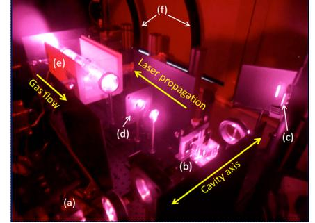
**Figure 1:** SEOP apparatus. (a) laser diode bar; (b) beam-splitter cube (1/3 feedback along cavity axis, 2/3 transmission along cell axis); (c) holographic grating; (d)  $\lambda/4$ -wave plate; (e) ceramic oven for housing cell (lid removed); (f)  $B_0$  coils
