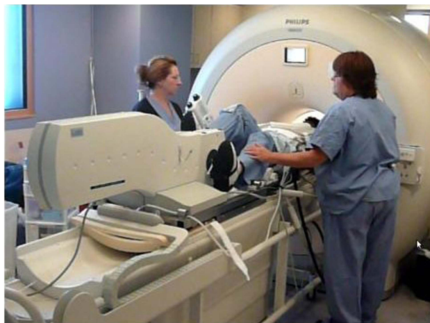
Figure 1. MR compatible supine exercise imaging apparatus mounted on the MR scanner at 1.5T.
