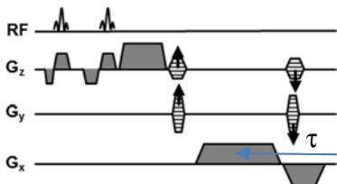
**Fig 1** Water-selective 3D SSFP-echo pulse sequence using two RF pulses separated by 1.196 ms at 3T. After the 2<sup>nd</sup> RF, a crusher dephases the FID and imparts additional phase to moving spins. Effective TE is approximately  $(2 \times TR) - \tau$ , i.e. the first echo is formed on the 2<sup>nd</sup> cycle of the pulse sequence.
