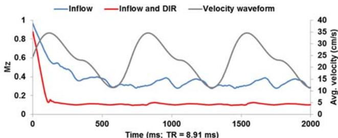
**Fig 2** Bloch equation simulation of blood longitudinal magnetization for SSFPe (blue) and DIR-SSFPe (red). For reference, simulated monophasic velocity waveform is also shown (gray).
