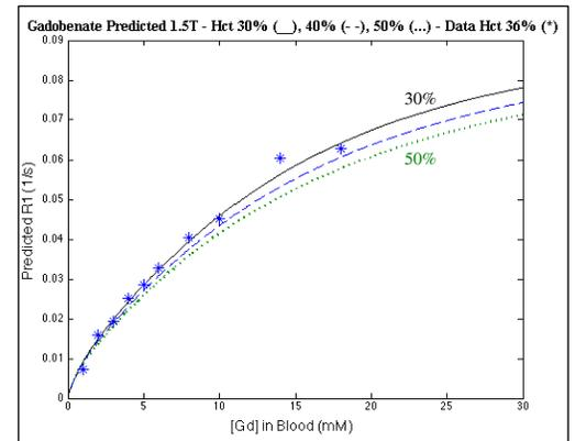
**Figure 1.**  $R_1$  vs. [Gd] at 1.5T; Gadobenate in blood. Predicted 2SX modeling demonstrating non-linearity  $R_1$  vs. [gadobenate] (deviation from linear line) and predicting some Hct dependence. Experimental data for Hct 36% matches well, validating model (similar excellent matching other GBCA at both  $B_0$ ).
