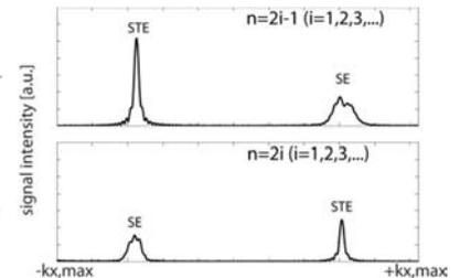
**Figure 2:** Two consecutive k-space lines (phase encoding was turned off during acquisition). The separated and differently weighted echo groups (spin echo (SE), stimulated echo (STE)) are clearly visible. Additionally, the change of position from one echo spacing to the next is demonstrated.
