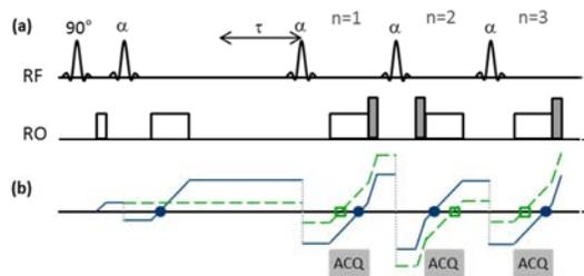
**Figure 1:** (a) Basic principle of the proposed two-in-one FSE, showing the radiofrequency pulses (RF) and the readout scheme (RO). An evolution time  $\tau$  is inserted after the first refocusing pulse. (b) The echo formation is shown for the spin echo (solid, blue line) and for the primary stimulated echo (dashed, green line). From the second echo spacing (ES) on two echoes occur: refocused spin echo (bold blue circle) and the refocused stimulated echo (open green square).
