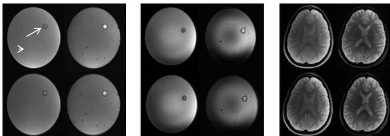
**Figure 3:** (left) Phantom images obtained at 3.0 T, (middle) phantom images measured at 7.0 T, (right) *in vivo* brain images of a healthy volunteer acquired at 3.0 T. For each subplot the upper row was reconstructed from a standard FSE sequence (left) and a  $T_2^*$  weighted FSE sequence (right) using the split approach [6]. The images in the lower row are generated by the proposed two-in-one sequence, producing both contrasts within one protocol.
