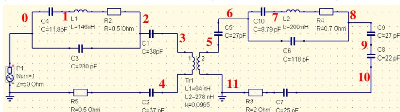
Fig. 1: Inductive feeding (left) and field generating loop (right)
