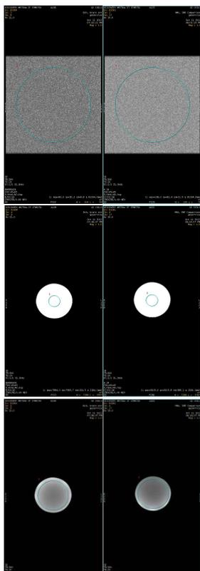
Fig.2: Axial Noise Images (Top) & Signal Images (Middle & Bottom) of a spherical phantom taken from 8 Channel Brain Coil (Left) and MR-PET HNU Coil (Right)
