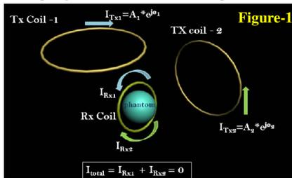
Figure-2: Experimental setup: Tx/Rx coils
