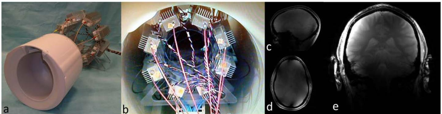
**Figure 1.** The 8 in-bore RF amplifiers are arranged on a circular former behind an 8 channel transmit / 32 channel receive coil. (a) The in-bore amplifiers are shown in operating position inside the bore of a 7T magnet. (b) FLASH images (1x1x5mm, TR/TE=150/4 ms) acquired with the in-bore amplifiers do not present any artifacts. (c-e)
