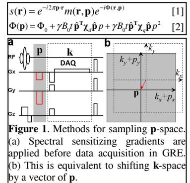
**Figure 1.** Methods for sampling **p**-space. (a) Spectral sensitizing gradients are applied before data acquisition in GRE. (b) This is equivalent to shifting **k**-space by a vector of **p**.
