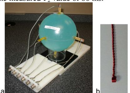
**Figure 1.** (a) A photograph of the eddy-current measuring apparatus. (b) A zoomed-in view of one of the solenoids that was immersed in the phantom.
