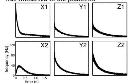
**Figure 2.** A typical time course of eddy currents for concatenated FIDs acquired at 10-ms intervals, for a total acquisition time of 1.8 s, after an impulse gradient was applied along the  $x$ -axis.
