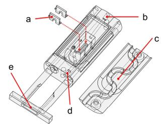
Figure 1: MRI compatible incubation chamber (exploded). Diameter 26mm. a) inserts & bench support the optic nerve, b) inflow, c) preheating system in lower section, d) outflow and e) isocenter positioning bar.
