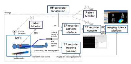
Fig. 1: MR-EP suite set-up with data exchange paths between components.
