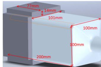
**Fig. 1:** The phantom (white), placed parallel to the z axis and four identical dielectric blocks (grey) of the same permittivity positioned around the bottle.
