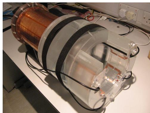
Figure 2 – The fully assembled waveguide. The four receive elements can be seen in the bottom-right of the image.
