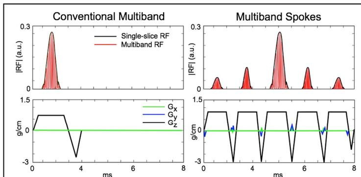
**Figure 2:** Illustration of conventional multiband and multiband spokes excitation RF and gradient waveforms. Also plotted are single-slice waveforms for comparison.
