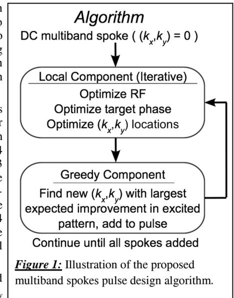
**Figure 1:** Illustration of the proposed multiband spokes pulse design algorithm.
