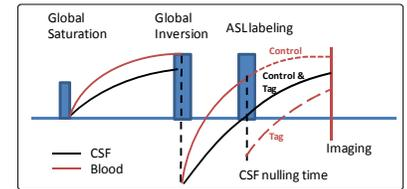
Fig. 1: CSF suppression strategy. The ASL labeling pulses are applied at the CSF signal nulling point: the CSF stays unlabeled while blood is regularly labeled. With such a scheme inflowing CSF should produce zero  $\Delta M$ .
