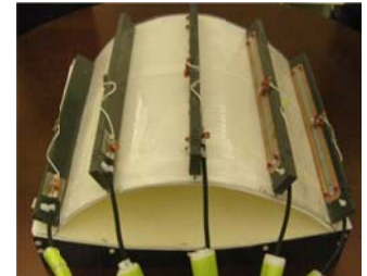
Fig.1 Photograph of 8ch mf-dipole array
