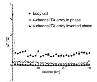
Fig 3:  $\Delta T$  along the wire from the tip (0 cm) to the phantom exit (30 cm)
