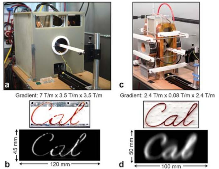
**Figure 1:** MPI scanners built in our lab already demonstrate millimeter-scale resolutions. (a) FFP and (c) Projection (FFL) MPI scanners. MPI images of “Cal” phantoms filled with 10x diluted Resovist SPIOs acquired with (b) FFP and (d) projection MPI scanners. Due to stronger magnetic field gradients, the image in (b) has 3x finer resolution than the image in (d).
