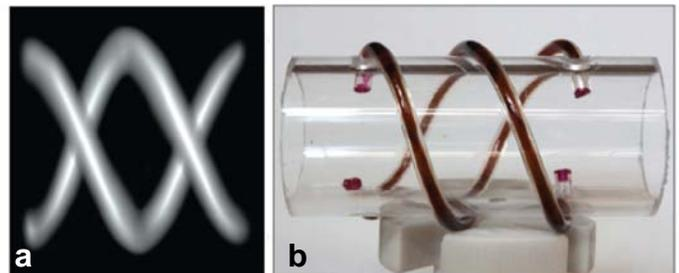
**Figure 2:** MPI image of a vasculature-mimicking helical phantom filled with undiluted Micromod nanomag-D SPIOs, acquired on our projection (FFL) MPI scanner. (a) Volume-rendered MPI image after 3D projection reconstruction of 40 projections. (b) Photo of the phantom (tubing ID: 1.6 mm). 2 min 7 s scan. FOV: 6 x 6 x 7.3 cm<sup>3</sup>.
