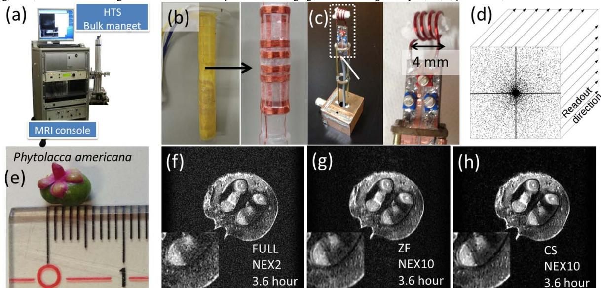
Fig. 1. (a) The MR microscope using the HTS superconducting bulk magnet. (b) A 3-axis gradient coil set. (c) A solenoid RF coil. (d) An undersampled Cartesian trajectory used in this study. (e) *Phytolacca americana* measured using our MRI system. (f-h) MR images reconstructed from (f) fully sampled k-space data and undersampled k-space data with (g) ZF and (h) CS.
