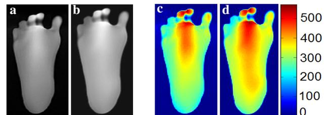
Fig 3. Axial images of foot phantom using FFCA are shown in (a) and (b) (FSE  $T_1$  and  $T_2$ ). The corresponding SNR maps of FFCA are shown in (c) and (d).
