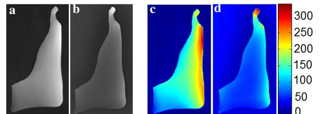
Fig 2. Sagittal image (FSE  $T_1$ ) of foot phantom using FFCA (a) and eight channels phase array head coil (b). The SNR maps of FFCA and eight channels phase array head coil are shown in (c) and (d).
