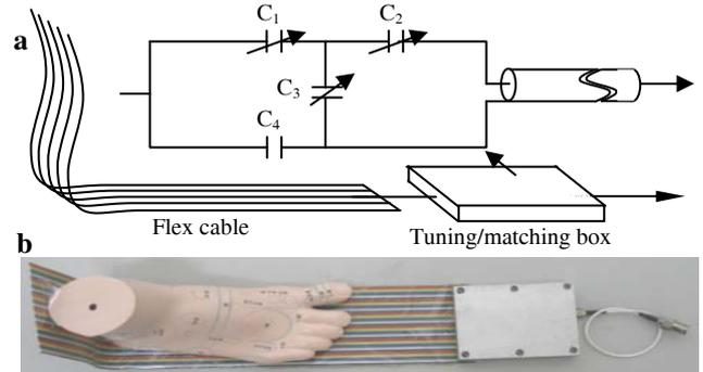
Fig.1 Schematic representation of the proposed FFCA (a) and the photo of FFCA with foot phantom.
