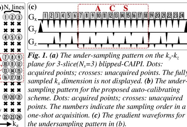
**Fig. 1.** (a) The under-sampling pattern on the  $k_y$ - $k_z$  plane for 3-slice ( $N_s=3$ ) blipped-CAIPI. Dots: acquired points; crosses: unacquired points. The fully sampled  $k_x$  dimension is not displayed. (b) The under-sampling pattern for the proposed auto-calibrating scheme. Dots: acquired points; crosses: unacquired points. The numbers indicate the sampling order in a one-shot acquisition. (c) The gradient waveforms for the undersampling pattern in (b).
