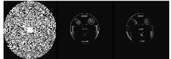
Figure 2. Left: Poisson-disc undersampling pattern with acceleration factor of 1.3 for each channel. Middle and right: Individual fully sampled channels from a 7 T scanner using a 2D GRE sequence (TR=250 ms, TE=3.2ms, 90° flip angle, 31.25 kHz bandwidth, 3 averages).
