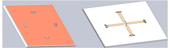
Figure 1. A 2-channel traveling wave transceiver array, fabricated on a teflon substrate as orthogonal copper-foil microstrip transmission line resonators, was used to acquire images for the parallel-imaging reconstruction experiments.
