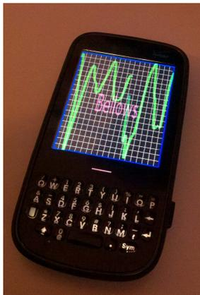
Figure 2: Real time respiration belt application. This app allows immediate feedback on the belt connection in a very portable form factor.
