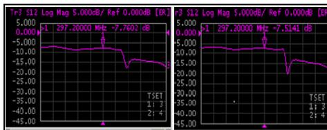
Fig. 2: Coupling between adjacent elements on a side in the 20-Ch Tx/Rx 7T modular head coil loaded with a human head. Left side is S34 of side 1 with all other sides and top are 2x2. Right side is the same with all other sides are 2x2 and top is 3x3.
