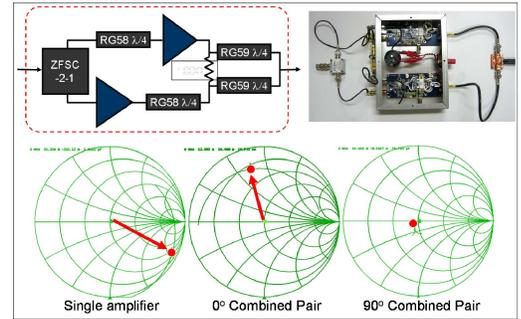
**Figure 1:** A 300MHz balanced implementation using output Wilkinson combiner and input 0 degree splitter creates 50Ω output port impedances.
