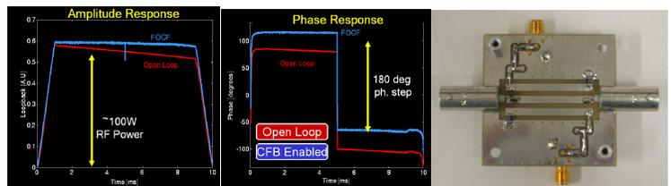
**Figure 2:** Cartesian feedback RF droop test of a 10ms trapezoidal rotary echo pulse. The power supply and capacitor voltage drop by 7 to 8 volts causing a subsequent RF amplitude droop and temporal phase drift for the open loop test (red). In comparison the CF linearized output (blue) is stabilized despite the power supply rail modulation. (Right) Mono-match bi-directional coupler for MR compatible power sensing.
