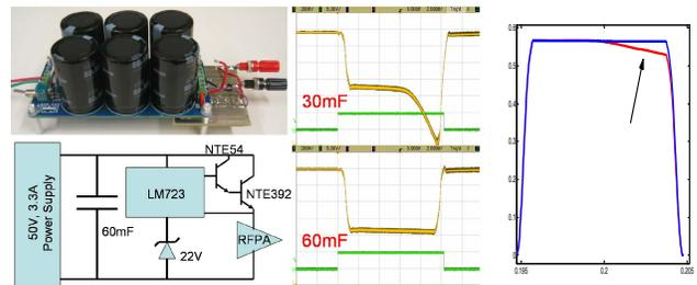
**Figure 3:** The pulse regulator system employs a 60mF capacitor bank and post-regulator with a Darlington transistor stage to stabilize the RF amplifier rails. The center scope shot shows the droop with inadequate (30mF) capacitors, and the right is the corresponding RF droop (red).
