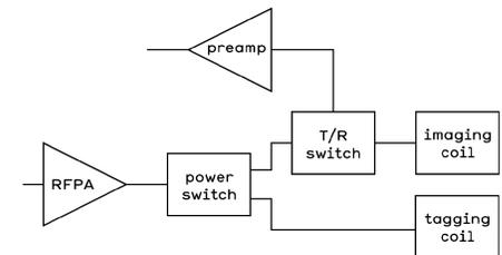
Figure 1: Block diagram showing the high power switch inserted before the T/R switch in the transmit pathway.
