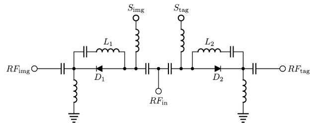
Figure 2: Circuit schematic.  $D_1$  and  $D_2$  are the PIN diodes,  $L_1$  and  $L_2$  resonate  $D_1$  and  $D_2$  in the off state. All remaining inductors are RF chokes ( $1\mu\text{H}$ ), all capacitors are DC blocks ( $620\text{pF}$ ).  $S_{\text{img}}$  and  $S_{\text{tag}}$  are the control signals.
