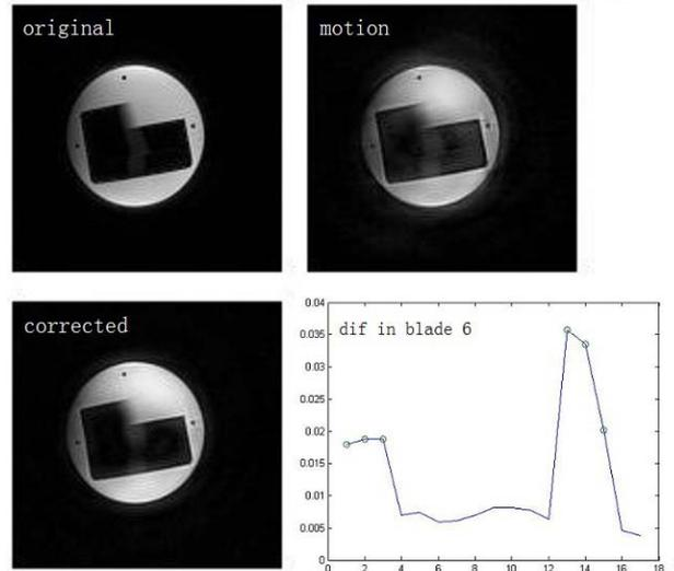
Fig.2 phantom results. In blade 6, lines 1 to 3, 13 to 15 are greatly larger than others as the result of introduced motion.
