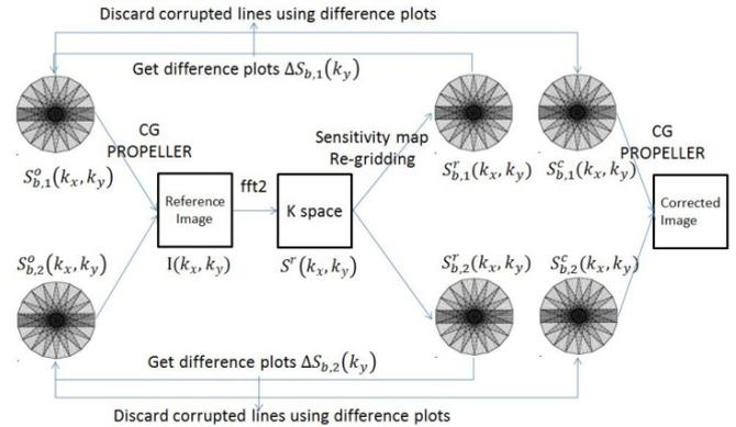
Fig.1 Schematic diagram of the proposed motion correction method
