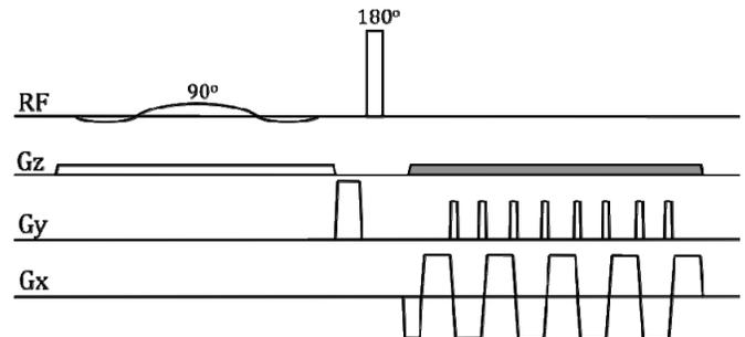
**Fig. 1** VAT-EPI sequence. Compared to standard EPI, there is an additional slice-axis gradient (shaded) applied during the entire readout period and the RF excitation pulse is elongated to reduce k-space modulation during the EPI readout.
