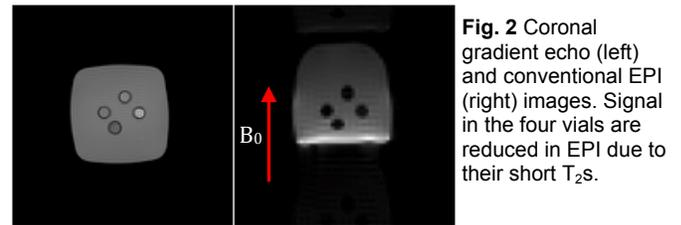
**Fig. 2** Coronal gradient echo (left) and conventional EPI (right) images. Signal in the four vials are reduced in EPI due to their short  $T_2$ s.
