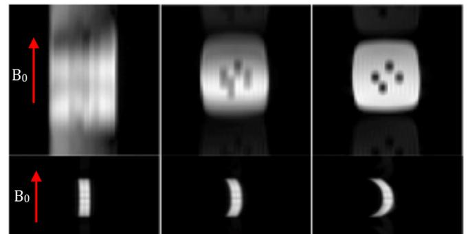
**Fig. 3** Coronal VAT-EPI images (top row) and corresponding slice profiles (bottom row) for excitation RF pulse widths, from left to right, 4.3, 18.7, 43.6 ms. For the slice profiles, a coronal slice-selective excitation was followed by a sagittal projection acquisition.
