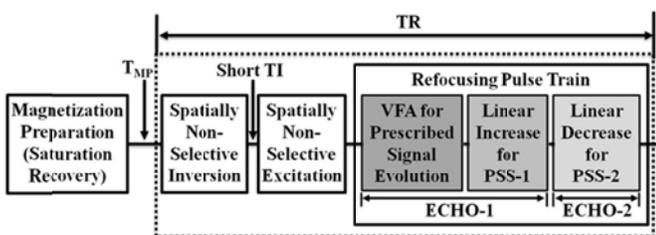
Fig. 1 A schematic of the proposed, dual-echo single-slab 3D turbo/fast spin echo pulse sequence for GM imaging.
