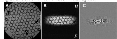
Figure 2: (a) Sagittal view through a cylinder phantom containing conical tubes. (b) The same sagittal view with current applied to ch. 1. (c) Real part of the image in (b) showing the contours of the magnetic field produced by the coil. Signal is localized predominantly in the cranial/caudal (H/F) direction due to ch. 1 geometry.
