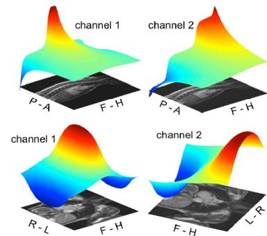
Figure 1: Magnetic field profiles (z-component) from 2 channels of the FlatLoc coil in the y-z (row 1) and x-z (row 2) planes of the magnet coordinate system overlaid on orthogonal views of the chest cavity (R-L, right to left, P-A, posterior to anterior, F-H, foot to head). The orthogonal fields allow spatial selection of anatomic shapes.
