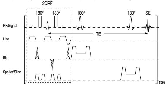
**Fig. 2:** Basic PRESS-based pulse sequence for MR spectroscopy using a segmented, “center-always” blipped-planar 2DRF excitation with three k-lines per segment. The middle one of the three lines covers the centre of k-space in each segment. Non-selective refocusing RF pulses were inserted between the k-lines to avoid chemical-shift displacement artifacts. One slice-selective refocusing RF pulse is used to eliminate side excitations in the blip direction.
