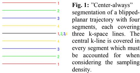
**Fig. 1:** “Center-always” segmentation of a blipped-planar trajectory with four segments, each covering three k-space lines. The central k-line is covered in every segment which must be accounted for when considering the sampling density.
