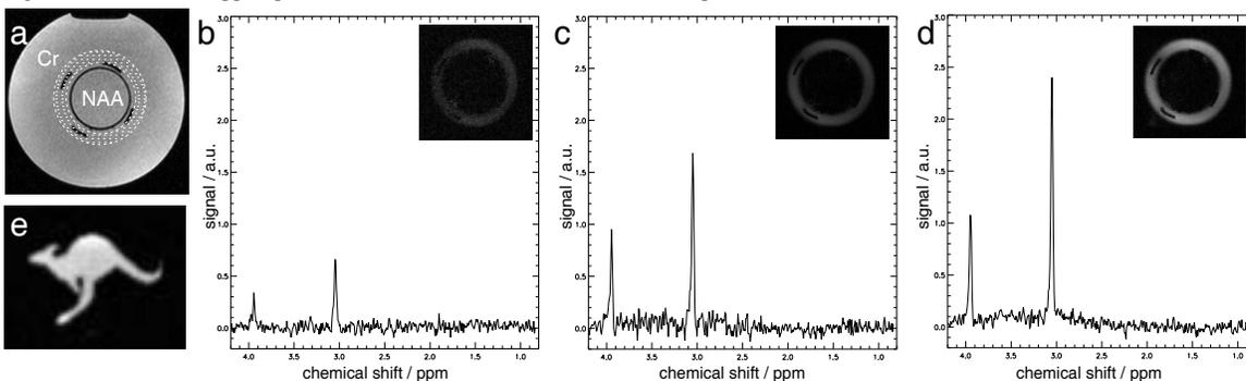
**Fig. 3:** (a) MR image of the spectroscopy phantom containing NAA in the inner and creatine in the outer bottle. (b-d) MR spectra and profile images acquired for the ring shaped ROI depicted in (a) with (b) single-line segments, (c) conventional multi-line segmentation, and (d) “center-always” multi-line segmentation. (e) Irregularly shaped excitation profile measured in an oil phantom with a “center-always” multi-line segmentation..
