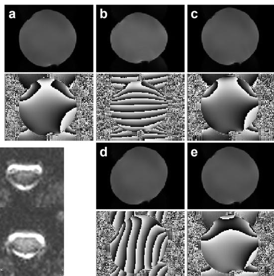
**Fig. 2:** Magnitude (upper) and phase images (lower) of a phantom for (a) optimized shim and (b-e) simulated field gradients in (b,c) phase encoding and (d,e) readout direction. (b,d) Without compensation, the phantom appears distorted, either (b) compressed or (d) sheared. (c,e) With appropriate additional pre-dephasing and blipped gradient pulses the distortions can be corrected
