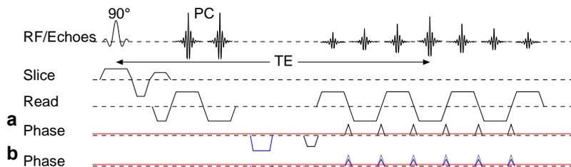
**Fig. 1:** Basic pulse sequence used in the present study for “y-shimming”. The red lines sketch a background field gradient in the phase-encoding direction that causes an echo time shift and geometric distortions. While the echo time shift can be compensated for (a) by a predephasing gradient pulse (blue), the geometric distortions require in addition (b) a modification of the blips (blue).
