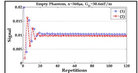
**Figure 2: Data taken in the empty 100mL phantom which shows how the signal level oscillates toward the steady state of (2-red) lower than (1-blue) due to the diffusion gradients.**
