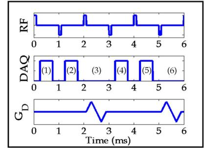
**Figure 1: SSFP with asymmetric attenuation through diffusion gradients.**
