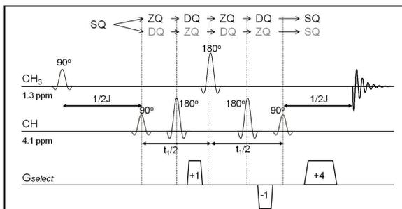
Figure 1; refocused double quantum selection sequence. The lactate signal is converted to a double quantum state where it is twice as sensitive to dephasing gradients. The overlapping (single quantum) lipid signal experiences asymmetric gradients and shows a reduced signal intensity, dependent on the effective spoiling area. The first excitation pulse was made slice selective to generate signal from a single slice.
