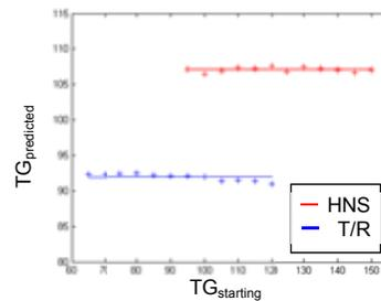
Figure 3:  $TG_{predicted}$  vs.  $TG_{starting}$  acquired with standard transmit/receive quadrature head coil (blue line) or with receive only 12-element head coil, body coil for transmission. The Bloch-Siegert shift method gives consistent results over a large range of starting TG setting.
