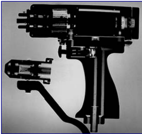
Figure 2: Prototype of the developed MR-compatible and x-ray transparent bone drill.
